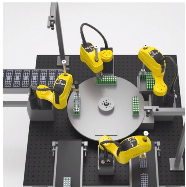
SR-3iA SCARA Robots assembling battery packs
